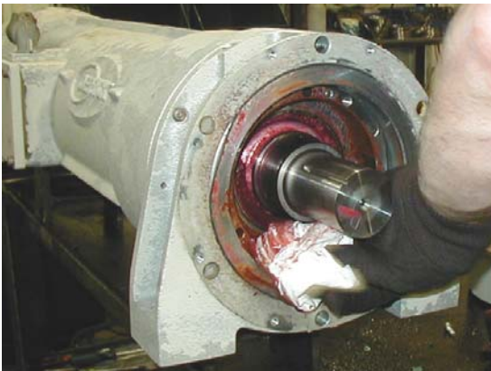
13 - Using a soft absorbent cloth, remove excess lubricant from interior of bearing housing and inner bearing race. Do not use compressed air for cleaning as this may drive contaminants into motor.
